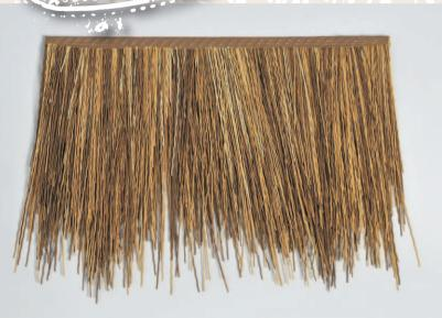
**Installation:** The grounding consists of complete roof being covered by wooden plates, then a complete sheeting in waterproof PE foil to which the Artificial Thatch is fixed with staples. The staples cross through the flexible top binder by staple gun, the stainless steel nails are also feasible.
